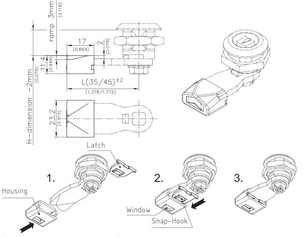
The Housing will be pushed onto the cam until it alines with the cam.
